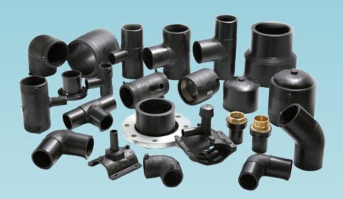
HDPE (High Density Poly Ethylene) pipes and fitting are available in complete range from 20 to 450 mm size. The pipes are available in PN 2.5 to PN 16 pressure class in PE 63, PE 80 and PE 100 grades. HDPE pipes are manufactured according to IS: 4984
